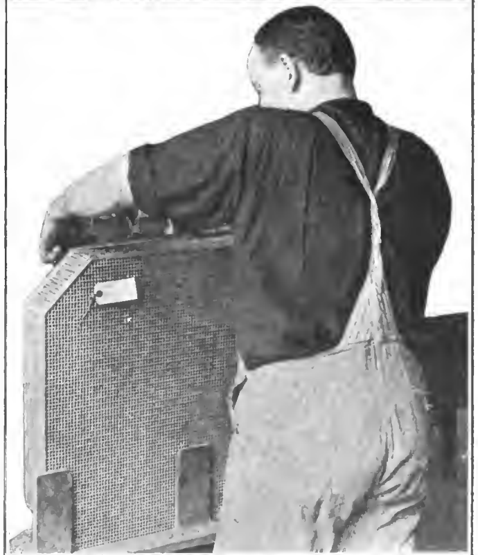
Stage 9—Fitting the radiator frame to the section before soldering them together
